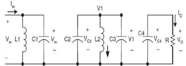
Fig. 6. Super Re-Lift circuit diagram during switch on period.
