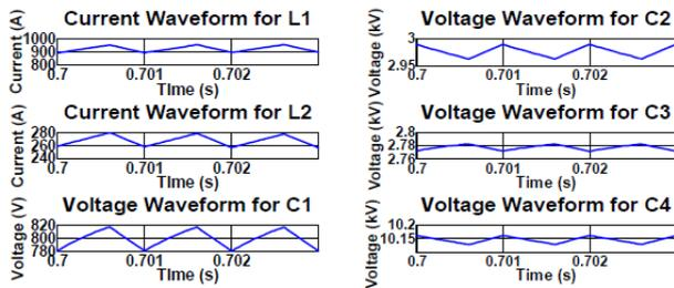
Fig. 9. Super Re-Lift inductor currents and capacitor voltages waveform with design criteria of input 1 kV and output 10 kV, at 1MW.
