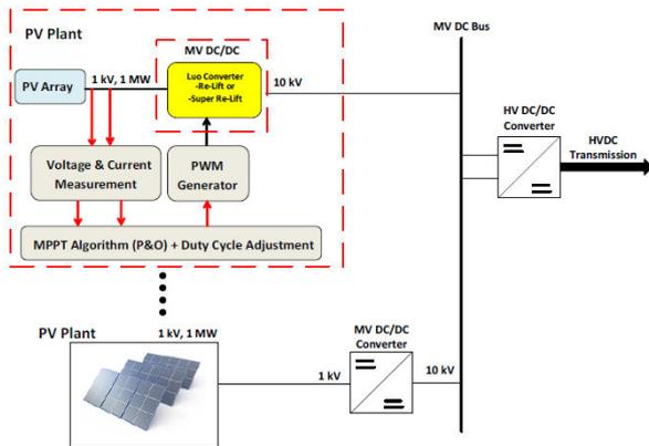
Fig. 1. General block diagram of the addressed MV DC network (1kV is assumed the voltage of the MPP of the installed PV).
