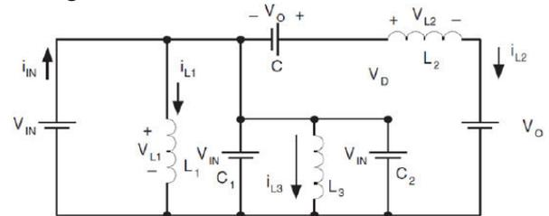
Fig. 3. Re-Lift circuit diagram during switch on period.
