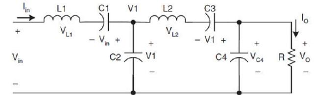
Fig. 7. Super Re-Lift circuit diagram during switch off period.
