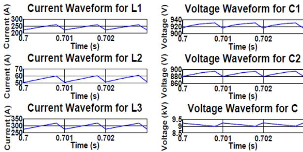
Fig. 8. Re-Lift inductor currents and capacitor voltages waveform with design criteria of input 1 kV and output 10 kV, at 1MW.
