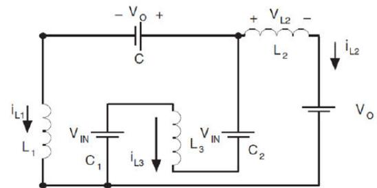
Fig. 4. Re-Lift circuit diagram during switch off period.
