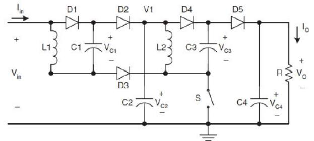
Fig. 5. Super Re-Lift circuit diagram.
